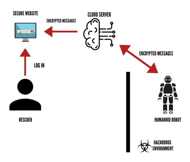
Figure 3.1: System architecture.
