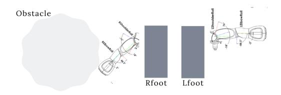
Figure 3.4: Detecting obstacles using hands.
