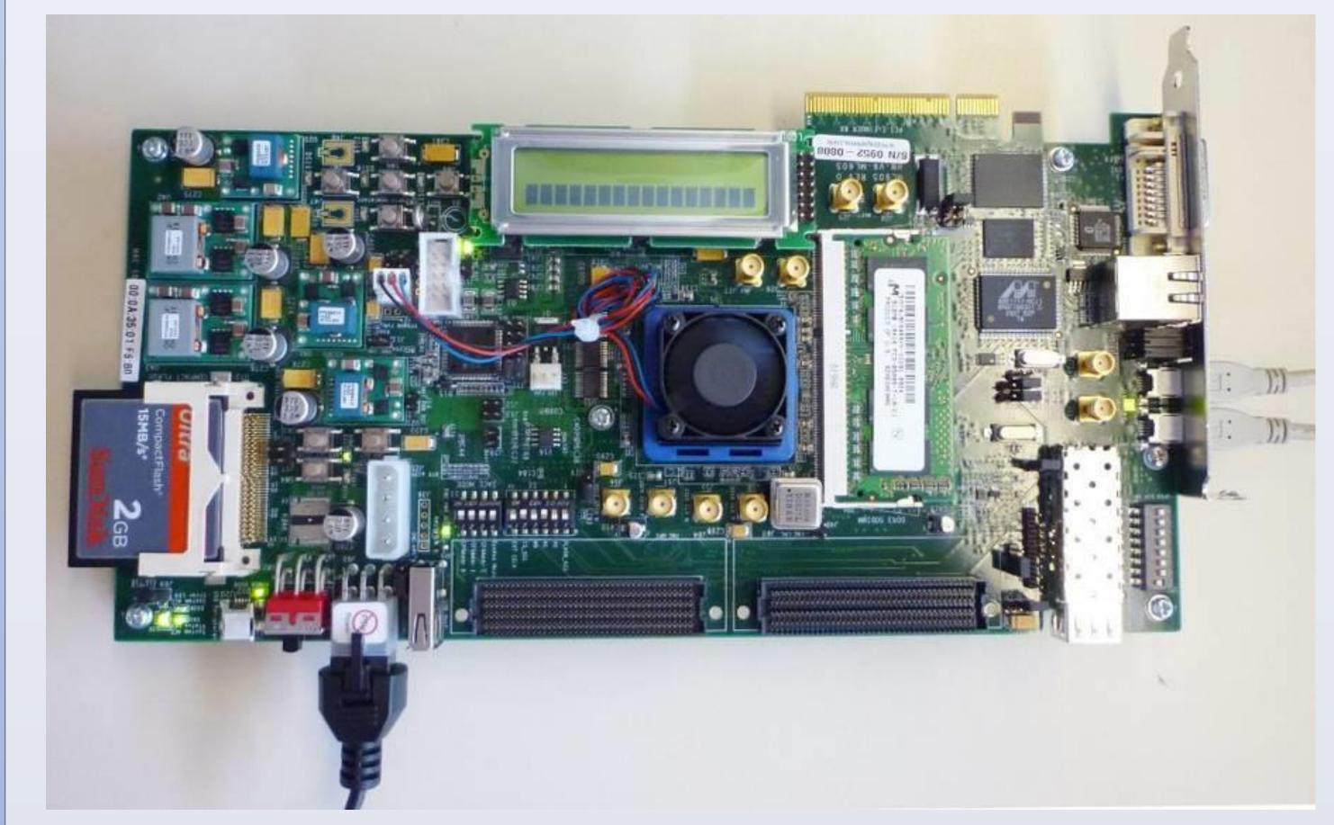
The Xilinx Virtex 6 ML605 FPGA Board that was used for the implementation
