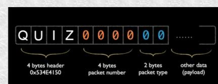
Multiplayer mode is based on Client-Server model. Data packets were used for messaging between devices. Finally, four state machines were created.
