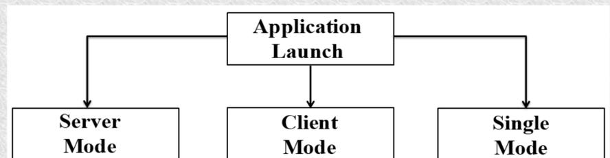
The flow diagram of user actions when starting the application. There are three options of execution. The first is about hosting an online-web game (server), and the second about a client in a network game. Finally, we have the function of single player.
